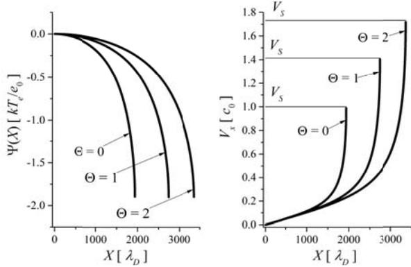
Figure 2: Potential  $\Psi(X)$  and velocity  $V_x(X)$  profiles obtained from the system (8) - (11), (16) for the parameters:  $K = 50$ ,  $Z = 2$ ,  $\alpha = 20^\circ$ ,  $\varepsilon = 10^{-4}$ ,  $\Theta = 0$ ,  $\Theta = 1$  and  $\Theta = 2$  and initial conditions (17) with  $V_0 = 10^{-8}$ .
