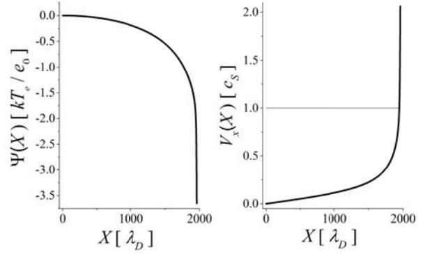
Figure 4: Potential  $\Psi(X)$  and velocity  $V_x(X)$  profiles obtained from the system (8) - (12) for the parameters:  $K = 50$ ,  $Z = 2$ ,  $\alpha = 20^\circ$ ,  $\varepsilon = 10^{-4}$ ,  $\Theta = 0$  and initial conditions (17) with  $V_0 = 10^{-8}$ .
