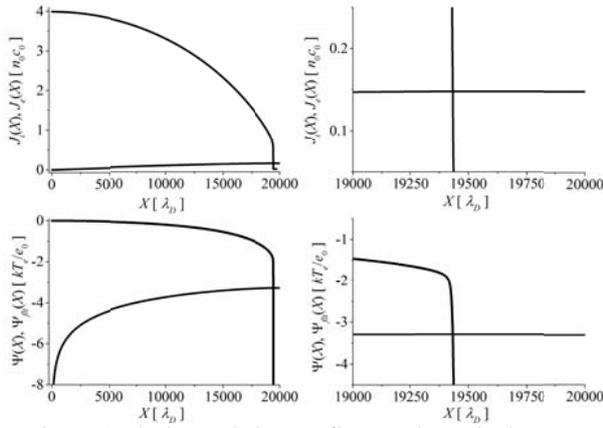
Figure 5: The ion and electron flux are shown in the top graphs. In the bottom plots the potential and the floating function are plotted. In the right plot a part of the respective left figure is shown on an expanded scale.
