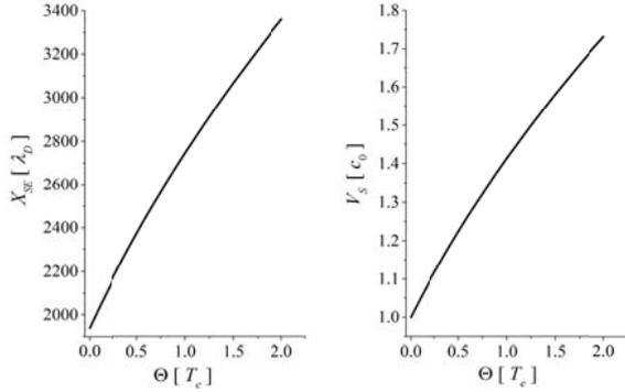
Figure 3: The sheath edge position  $X_{SE}$  and the ion sound velocity  $V_s$  versus  $\Theta$ .
