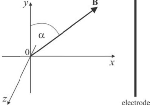
Figure 1: Schematic of the model. The magnetic field lies in the  $xy$  plane and the  $x$  axis is perpendicular to the electrode.
