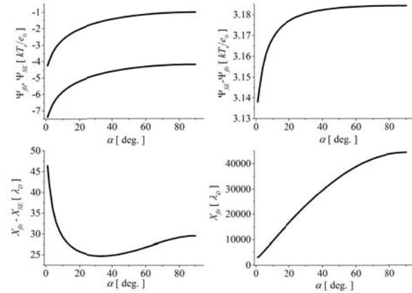
Figure 6: The floating and the sheath edge potential (top left), the sheath potential drop (top right), the sheath thickness (bottom left) and the electrode position (bottom right) versus the magnetic field angle  $\alpha$ .
