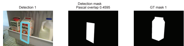
Figure 6: Occluded object detection. Detection is robust even though almost the whole bottom half of the object is occluded.
