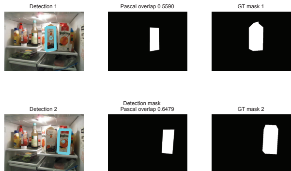
Figure 5: Object detection example. Our proposed method is able to detect an object from multiple views as well as detect multiple instances of the same object.
