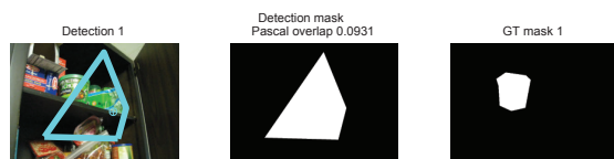
Figure 7: False detection. An object is falsely detected due to single keypoint voting. Since a large green area is found in the scene, which is the same colour as the object in question "potroastsoup", arbitrary keypoint detections appear which are matched to the object model.
