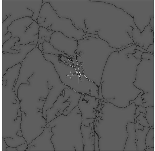
Figure 3: Reference roads within a search area. Pixel values correspond to the reference road feature map values  $G_{i,j}$ . Estimated location of the GCP is shown as bright cross, and white pixels represent rotated road patch  $P$  at its estimated location.
