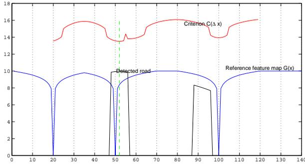
Figure 6: Simulation of the scaling and rotation errors (scenario B). The length between first and second detected road (right) is not the same as between reference roads, which leads to location estimation error.
