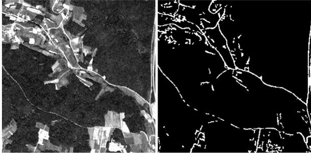
Figure 2: Satellite image patch (left) and corresponding detected road mask  $M$  (right).
