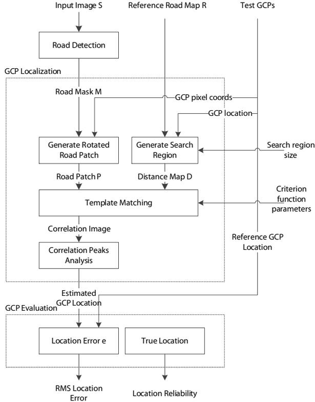
Figure 1: GCP extraction and evaluation algorithm.
