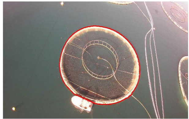
Fig. 7. Cage detected using joint angle and radius information
