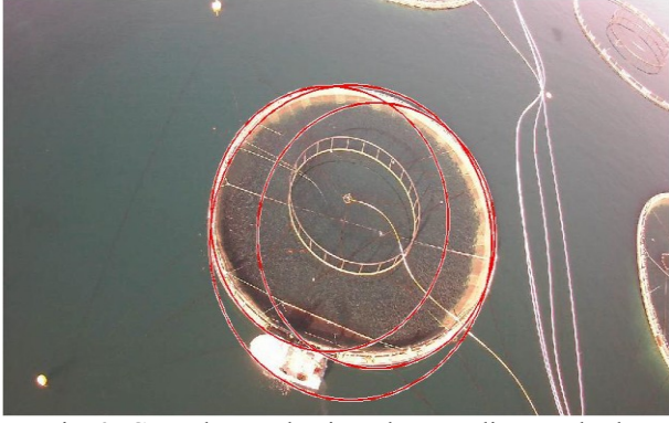
Fig. 3. Cage detected using phase coding method
