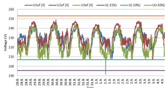
Figure 3 Effective voltage values without connected power plant
