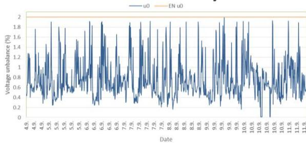
Figure 9 The negative sequence unbalance component with connected PV power plant
