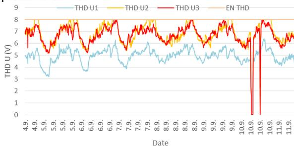
Figure 11 Total harmonic distortion of the voltage of phases L1, L2, and L3 with connected PV plant
