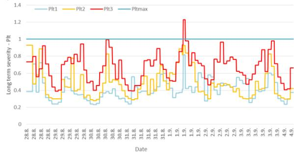
Figure 7 Diagram of long-duration voltage flickers with no connected PV power plant
