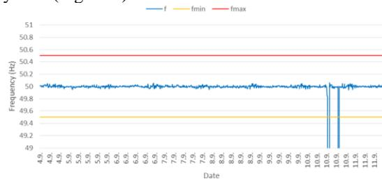
Figure 6 Frequency values with connected PV power plant
