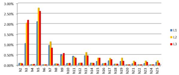
Figure 12 Amplitudes of higher-harmonic components with connected PV power plant
