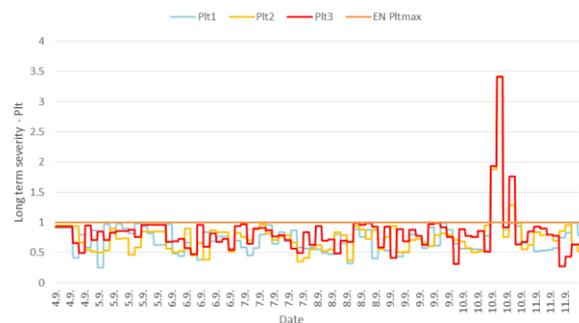
Figure 8 Diagram of long-duration voltage flickers with connected PV power plant
