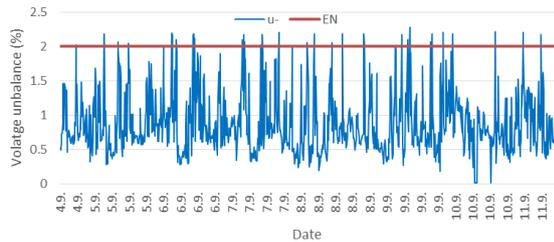
Figure 10 The zero-sequence unbalance component with connected PV power plant
