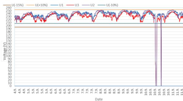
Figure 4 Effective voltage values with connected PV power plant
