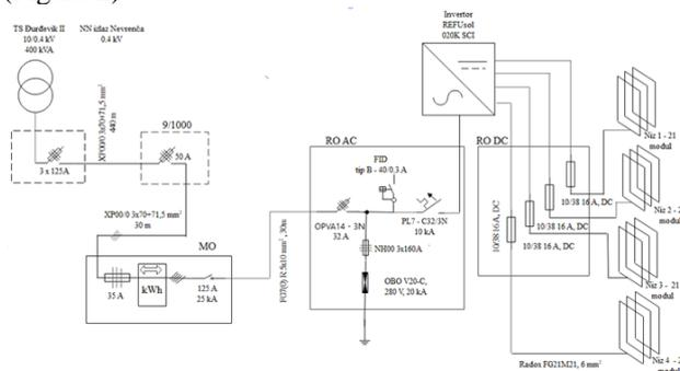
Figure 2 Single-plane scheme of the PV power plant
