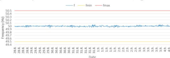
Figure 5 Frequency values with no connected PV power plant
