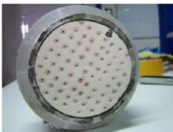
Figure 3: Ceramic specimen inside the Kundt tube sample holder
