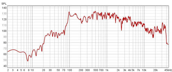
Figure 16. Frequency response of an acoustic guitar with a VIBE 1 microphone.
